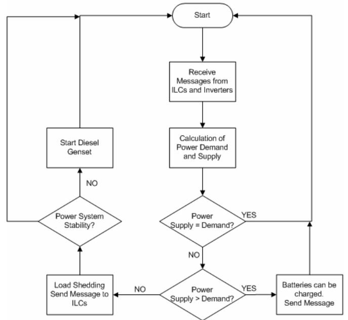
Fig. 5. Flow Chart of the MGCC Algorithm
