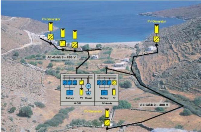
Fig. 2. The Kythnos Island Pilot Microgrid
