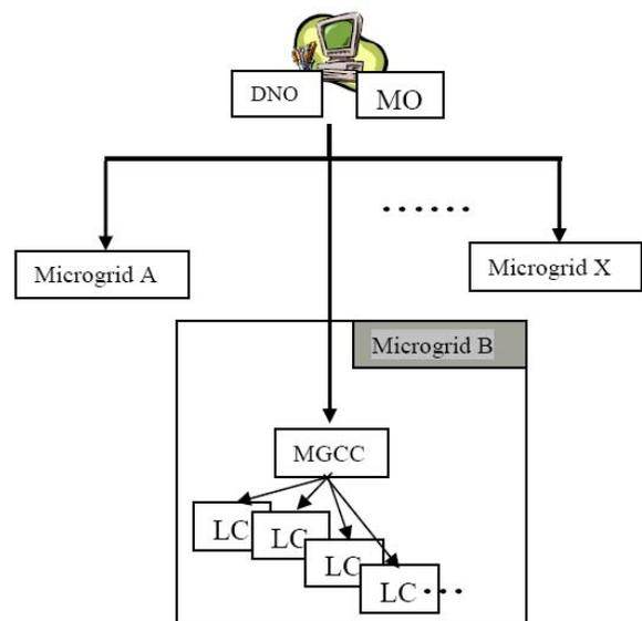
Fig. 1. Control levels of the Microgrid environment
